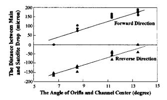
Figure 4. The Relationship Angle between orifice and channel center versus Distance between main and satelite dot on a printed matter.
